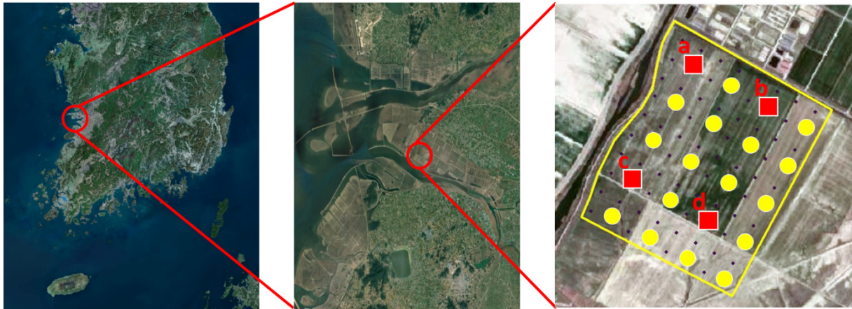
Fig. 1. Location of experimental site in Saemangeum reclaimed tideland. 20 point indicates the fields with variance spots in experimental site. In a right figure, the red squares indicate the locates installed sensor for monitoring groundwater levels and soil water contents. The a, b, c and d indicates the fields with different groundwater levels and soil water contents in experimental stations (a and b: stations of intermediate and shallow groundwater level, c and d: stations of deep groundwater level).
